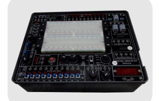
**DTK-01A** is a Single Board Trainer Kit which is widely used to train engineers to Develop/Study hardware for any Digital / Analog components in laboratory. This board has the provision for bread board which facilitates experimenting the Digital / Analog component Circuits.
