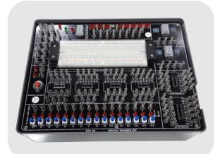
**DTK-09** is a Single Board Trainer Kit which is widely used to train engineers to Develop/Study hardware for any Digital components in laboratory. This board has the provision for bread board which facilitates experimenting the Digital component Circuits.
