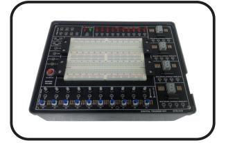
**DTK-01D** is a Single Board Trainer Kit which is widely used to train engineers to Develop / Study hardware for any Digital components in laboratory. This board has the provision for bread board which facilitates experimenting the Digital component Circuit.
