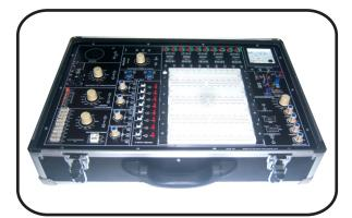
DTK-06 is a single board Breadboard Trainer Kit which is widely used to train engineers to develop/ Study hardware for any Digital/Analog integrated circuit in laboratory. This board having logic inputs, output indicator LED's, Push Switch Key, Sine/ Square wave Generator, Potentiometer, Panel Meter, General purpose Breadboard, AC/DC Supplies for experimenting the digital/analog techniques. In this board all interfacing between onboard source & breadboard are done by patch chords.
