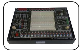
**DTK-08A** is a single board Digital Electronics Trainer Kit which is widely used to train engineers to develop/ Study hardware for any digital integrated circuit in laboratory. This board having logic inputs, output indicator LED's, Logic pulser, Clock Generator, Potentiometer, Seven segment display, General purpose Breadboard, DC Supplies for experimenting the digital techniques. In this board all interfacing between onboard source & breadboard are done by patch chords.
