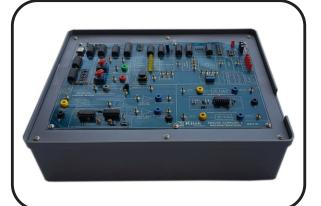
ACT-XX is a Digital Communication Trainer System to under stand various digital Modulation and Demodulation Techniques. Various functional block diagrams are provided on-board for Teaching/Training. This Kits provides with various Test Points to visualize the signals on Oscilloscopes.
