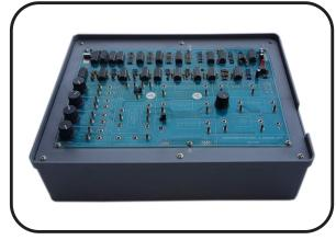
ACT-XX is a Digital Communication Trainer System to under stand various digital Modulation and Demodulation Techniques. Various functional block diagrams are provided on-board for Teaching/Training. This Kits provides with various Test Points to visualize the signals on Oscilloscopes.
