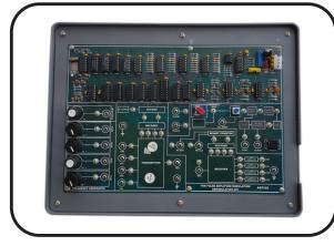
ACT-XX is a Digital Communication Trainer System to under stand various digital Modulation and Demodulation Techniques. Various functional block diagrams are provided on-board for Teaching/Training. This Kits provides with various Test Points to visualize the signals on Oscilloscopes.
