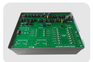
ACT-XX is a Digital Communication Trainer System to under stand various digital Modulation and Demodulation Techniques. Various functional block diagrams are provided on-board for Teaching/Training. This Kits provides with various Test Points to visualize the signals on Oscilloscopes.
