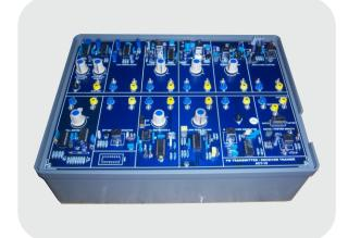
**ACT-10** is a Analog Communication Trainer System to under stand FM Modulation & Demodulation Techniques. Various Test points/ functional block diagrams are provided on-board for Teaching/Training.
