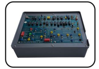
**ADCT-XX** is an Advance Digital Communication Trainer System that helps one under stand various Digital Modulation and Demodulation Techniques. Various functional block diagrams are provided on-board as an aid for Teaching/Training. These Kits are provided with various Test Points to visualize the signals on Oscilloscopes.
