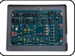
ADCT-XX is an Advance Digital Communication Trainer System that helps one under stand various Digital Modulation and Demodulation Techniques. Various functional block diagrams are provided on-board as an aid for Teaching/Training. These Kits are provided with various Test Points to visualize the signals on Oscilloscopes.
