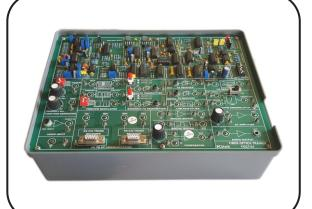
**FOCT-01** is a single board Fiber Optic Trainer Kit to study the characteristics of Fiber using Digital and Analog techniques. This kit also facilitates with digital and analog Modulation & Demodulation communication techniques.
