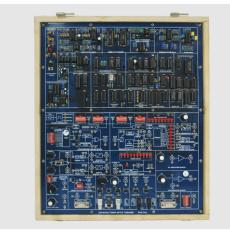
FOCT-02 is a single board Fiber Optic Trainer Kit to study the characteristics of Fiber using Digital and Analog techniques. This kit also facilitates with digital and analog Modulation & Demodulation communication techniques.
