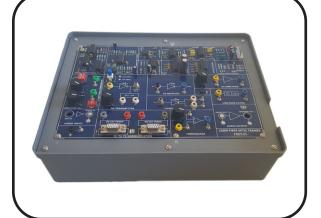
**FOCT-03** is a single board Laser Fiber Optic Trainer Kit to study the characteristics of Laser Fiber using Digital and Analog techniques. This kit also facilitates with PC to PC communication using RS-232C.
