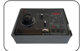
DC position control system is very use full in Controls System Laboratory . This system is easily understood and has a second order transfer function in the standard form, for which a well developed theoretical treatment is available.
