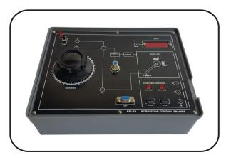
A.C. Position Control System is use full in control laboratory experiment. 2-phase ac servomotors have been traditionally used for position/ speed control applications especially in light weight, precision instrumentation area in airborne systems. The present unit is designed around a 12V ac servomotor and exposes the basic characteristics and dynamics of a position control system.
