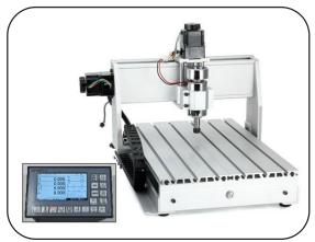
A small table top 3 Axis CNC Router kit which can cut, engrave or drill materials like Plastics, PCBs, Carbon Fibre and light metals like copper and brass. Working area of the machine is 290x390x65mm(X,Y,Z). It comes with a DC spindle with ER11 collet and can go upto 12000rpm. This model comes with 10/22Kg.Cm Hybrid Servo motors which give high rapid speeds upto 2500rpm.
