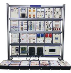
**KEE-02** Electrical Home Installation Trainer is a rouged training system for the Electrical laboratories mounted on Aluminum profile rack with sturdy table top flat panel. Each panel has ABS molded plastic sturdy enclosure with 4mm shrouded connectors showing circuit diagram & its connection tag numbers for easy understanding and connections. The product helps you to get fully acquainted with the basic concepts and functioning of an Electrical Machines & Generator.
