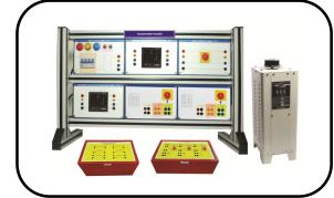
KEE-05 Power Transmission Line Trainer is a rouged training system for the Electrical laboratories mounted on Aluminum profile rack with sturdy table top flat panel. Each panel has ABS molded plastic sturdy enclosure with 4mm shrouded connectors showing circuit diagram & its connection tag numbers for easy understanding and connections. The product helps you to get fully acquainted with the basic concepts and functioning of a Power Transmission Line Trainer.
