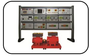
KMG-05 Electrical power Generation set up is a rouged training system for the Electrical laboratories mounted on Aluminum profile rack with sturdy table top flat panel. Each panel has ABS molded plastic sturdy enclosure with 4mm shrouded connectors showing circuit diagram & its connection tag numbers for easy understanding and connections. The product helps you to get fully acquainted with the basic concepts and functioning of a Electrical power Generation set up
