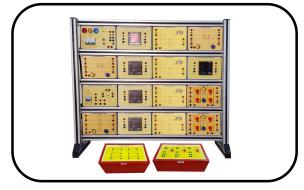
KMG-07 Double Bus Bar Trainer is a rouged training system for the Electrical laboratories mounted on Aluminum profile rack with sturdy table top flat panel. Each panel has ABS molded plastic sturdy enclosure with 4mm shrouded connectors showing circuit diagram & its connection tag numbers for easy understanding and connections. The product helps you to get fully acquainted with the basic concepts and functioning of a Double Bus Bar Trainer.
