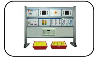
KPR-06 Distance Protection Relay Trainer Is a rouged training system for the Electrical laboratories mounted on Aluminum profile rack with sturdy table top flat panel. Each panel has ABS molded plastic sturdy enclosure with 4mm shrouded connectors showing circuit diagram & its connection tag numbers for easy understanding and connections. The product helps you to get fully acquainted with the basic concepts and functioning of a Distance Protection Relay Trainer
