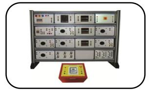
KPR-12 Feeder Protection Relay Trainer is a rouged training system for the Electrical laboratories mounted on Aluminum profile rack with sturdy table top flat panel. Each panel has ABS molded plastic sturdy enclosure with 4mm shrouded connectors showing circuit diagram & its connection tag numbers for easy understanding and connections. The product helps you to get fully acquainted with the basic concepts and functioning of a Feeder Protection Relay Trainer.
