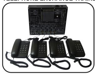
KVT-02 TELEPHONE EXCHANGE TRAINER is a Microprocessor based system designed to help the students to understand the basic concept and working of a Telephone Exchange. All the components are mounted on a single PCB in functional blocks and have various Test points to monitor all kinds of telephonic signals.
