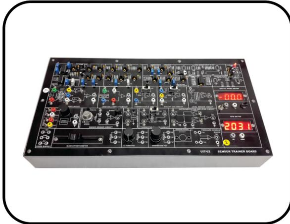
**UIT-02** is a Sensor Trainer offer Complete training opportunity for most commonly used Sensor available for experimenting in the Laboratory. Due to the typical Strength obtain from a sensor is not enough to process the signal; this board provides signal conditioners with Digital panel meter for display.
