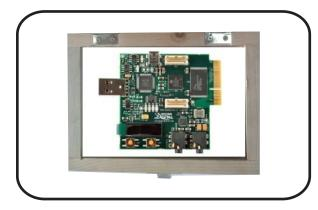
TMS320V5515 is a single board DSP Trainer Kit which is widely used to train engineers to develop on software/hardware for any communication applications control. Kit has power-full Monitor Includes Flash Memory, Stereo codec, OLED, Push switch, USB for Man to Machine Interface.
