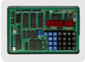
**M51-01** is a single board Microcontroller Trainer Kit based on 8 bit 8051 Microcontroller, which is widely used to train engineers to develop on software/hardware for any industrial process & control. Kit has power-full Monitor EPROM, RAM, I/O Lines, Timer/Counter, Serial, Seven Segment Display, Keyboard for Man to Machine Interface.
