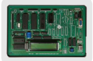
M51-02 is a single board Microcontroller Trainer Kit based on 8 bit 8051 Microcontroller, which is widely used to train engineers to develop on software/hardware for any industrial process & control. Kit has power-full Monitor EPROM, RAM, I/O Lines, Timer/Counter, Serial, LCD Display, Keyboard for Man to Machine Interface.
