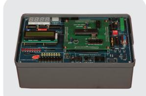
**E87-04** is a single board Universal Embedded Kit based on AVR (ATMEL Atmega32) Microcontroller for any Embedded applications.
