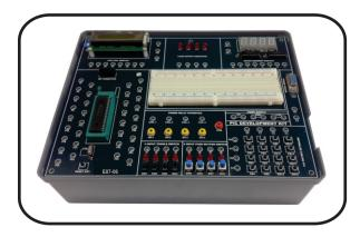
E87-03 is a single board Universal Embedded Kit based on PIC (Microchip 16F877A/ 18F452) Microcontroller for any Embedded applications.
