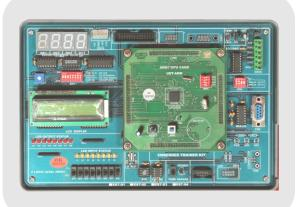
**E87-02** is a single board Universal Embedded Kit based on ARM (Philips LPC2148 / LPC2378) Microcontroller for any Embedded applications.
