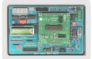
**E87-01** is a single board Universal Embedded Kit based on MCU (Philips 89C61X2 / P89V51RD2) Microcontroller for any Embedded applications.
