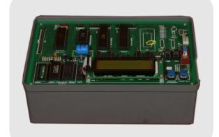
M85-04 is a single board Microprocessor Trainer Kit based on 8085 Microprocessor, which is widely used to train engineers to develop software/hardware for any industrial process & control. This Kit consists of power-full Monitor EPROM, RAM, I/O Lines, Timer/Counter, Serial, 20x2 LCD Display and Keyboard for Man to Machine Interface.
