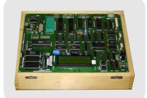
M85-07 is a single board Microprocessor Trainer Kit based on 8085 Microprocessor, which is widely used to train engineers to develop software/hardware for any industrial process & control. This Kit consists of power-full Monitor EPROM, RAM, I/O Lines, Timer/Counter, Serial, 16x1 LCD Display and Keyboard for Man to Machine Interface.
