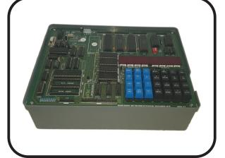
M86-01 is a single board Microprocessor Trainer Kit based on 16 bit 8086 Microprocessor, which is widely used to train engineers to develop software/hardware for any industrial process & control. This Kit consists of power-full Monitor EPROM, RAM, I/O Lines, Timer/Counter, Serial, Seven Segment Display and Keyboard for Man to Machine Interface.
