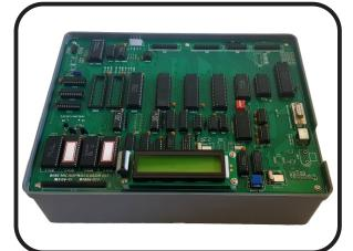
M86-02 is a single board Microprocessor Trainer Kit based on 16 bit 8086 Microprocessor, which is widely used to train engineers to develop software/hardware for any industrial process & control. This Kit consists of power-full Monitor EPROM, RAM, I/O Lines, Timer/Counter, Serial, LCD Display and Keyboard for Man to Machine Interface.
