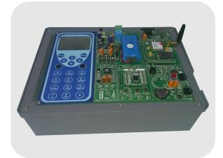
ACT-17 GSM Mobile Trainer Kit is an easy medium of learning the fundamental concept of Mobile communication like GSM, GPRS. The main focus of MCLS is in opening up a whole new world for you, mobile communication concepts like Call setup, call forward, SMS, voice, data and other Network protocols are also experimented on vis-à-vis the existing environment.
