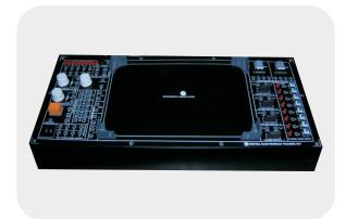
KMS-01B is Versatile trainer which is capable of performing the role of Linear/Digital IC Trainer, Gates, Flip flop, synchronous, ADC, DAC, Decoder, Multiplexer, Eprom, RAM, FPGA, CPLD, Basic Electronics Trainer, network circuit & theorms trainer, rectifier, filter & regulator trainer, Transistor amplifier circuits trainer, oscillator & waveshaping circuits trainer, linear circuits trainer, electrical bridges trainer, power electronics trainer and digital electronics trainer.
